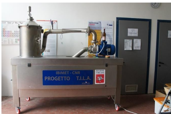
Picture 1. Pilot plant brewing by hydrodynamic cavitation
